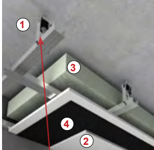
Typical application of sound insulating gypsum board ceilings
