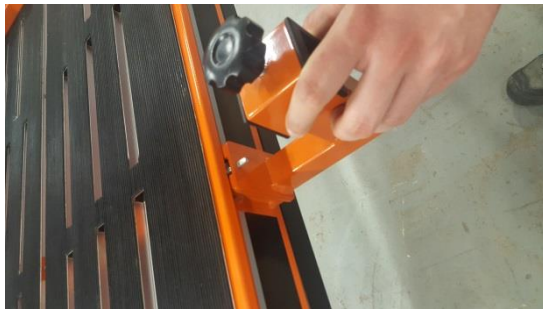
Insert both guide supports and lock them with knobs
