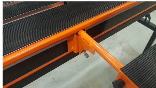
Rotate both shafts by 90° to lock side extension
