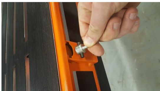
Insert 2 threaded and pinned shafts
