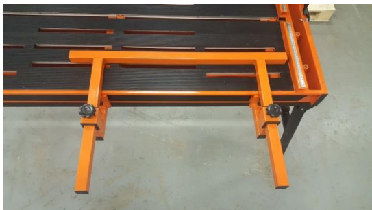
Insert the guide in both supports
